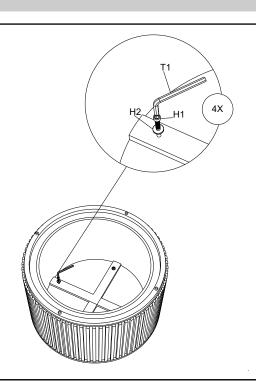
Place the MarbleTop (B) upside down position onto a padded non-marring surface. Align the hole of Marble Top(B) with pre-drilled holes underneath Wooden Base (A) and secure connection using Allen Bolts (H-1) and Flat Washer (H-2) with the help of Allen Key (T-1). Adjust overhang of Marble Top (B) with Wooden Base (A). Now fully tightened all Bolts.
